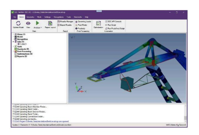
SDC Verifier is a software that verifies structures according to different design rules or codes. It works independently or on top of Ansys, Femap and Simcenter.
