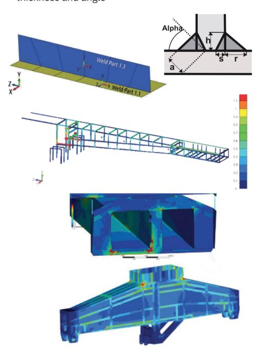
It is also possible to run Fatigue checks using **Hot Spot Stress Method**. Reference point settings are based on **IIW Fatigue Recommendations IIW-1823-07/ XIII-2151r4-07/XV-1254r4-07 Dec. 2008:**
