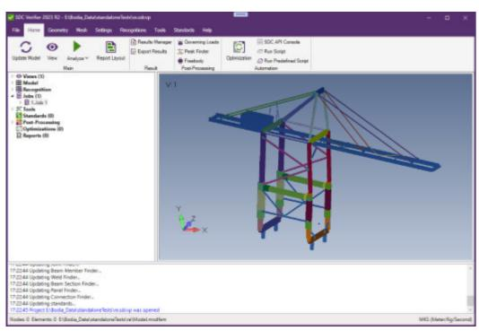
SDC Verifier is a software that verifies structures according to different design rules or codes. It works independently or on top of Ansys, Femap and Simcenter.
