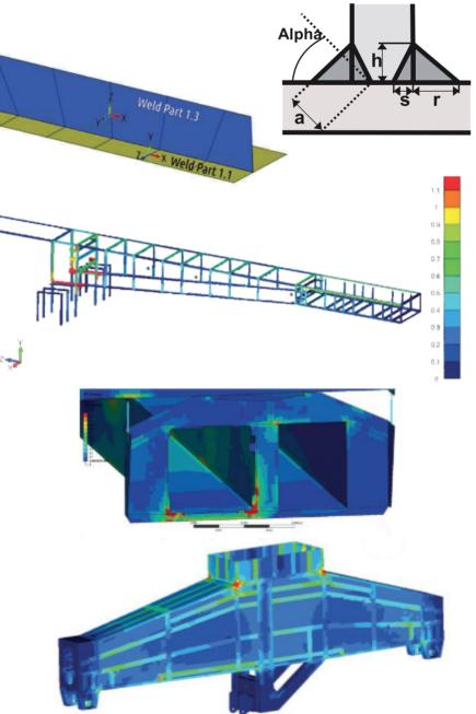
It is also possible to run Fatigue checks using Hot Spot Stress Method. Reference point settings are based on **IIW Fatigue** Recommendations IIW-1823-07/ XIII-2151r4-07/XV-1254r4-07 Dec. 2008:
