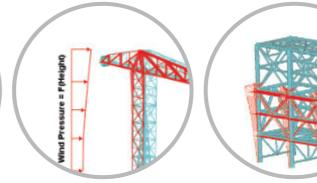
Wind – height dependent pressure applied to the model taking into account the element area exposed to the wind direction.
