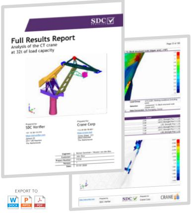
**Report Designer** is an advanced tool for automatic reports generation. Reports in SDC Verifier have a template-based structure and contain model setup, model description, and calculated results presented as plots and tables. In case of any changes in the analysis process, all results could be regenerated with one click.
